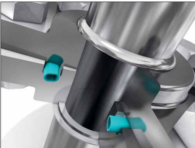
Figure 11 Example of Wills Rings® with its groove
