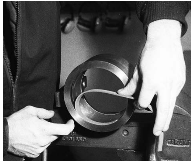
Figure 154 Installing Captive Slydring®
